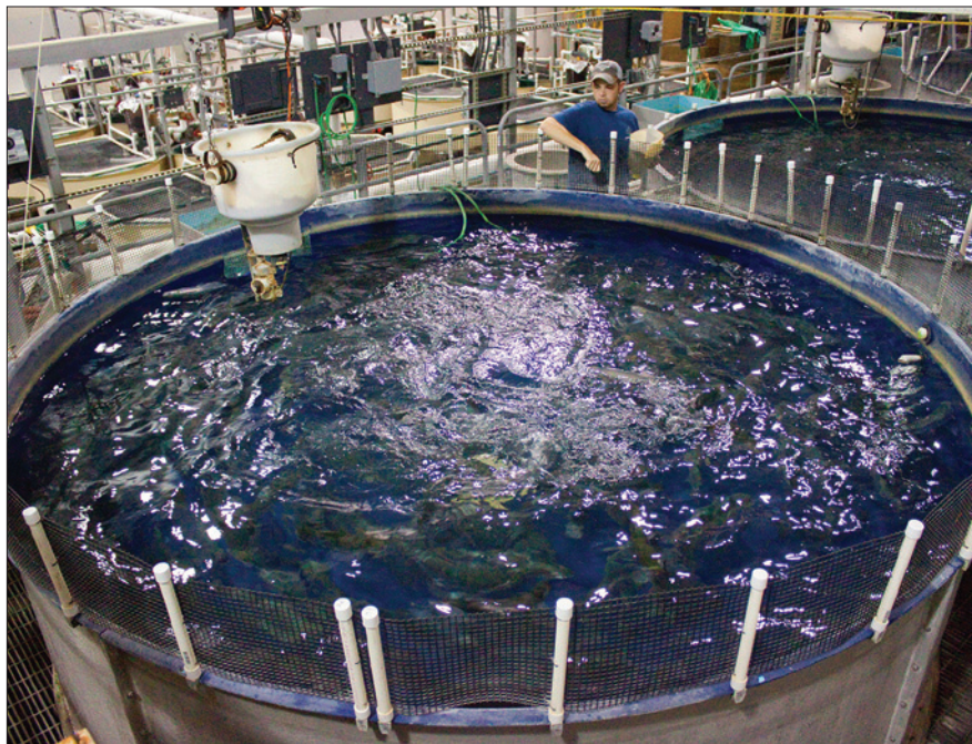
In ASF's joint project, the Atlantic salmon are grown in tanks at the Freshwater Institute's facility in West Virginia. Wastes are collected, and water is recirculated. There has been no need for antibiotics in the growth process.
